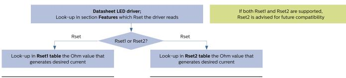
Note on E-series: in electronics, international standard IEC 60063 defines preferred number series for amongst others resistors. It subdivides the interval between subsequent values from 1 to 10 into 6, 12, 24, 48, 96 etc. steps. These subdivisions ensure that when some arbitrary value is replaced with the nearest preferred number, the maximum relative error will be on the order of 20%, 10%, 5%, 1% etc.
