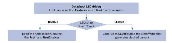
Note on E-series: in electronics, international standard IEC 60063 defines preferred number series for amongst others resistors. It subdivides the interval between subsequent values from 1 to 10 into 6, 12, 24, 48, 96 etc. steps. These subdivisions ensure that when some arbitrary value is replaced with the nearest preferred number, the maximum relative error will be on the order of 20%, 10%, 5%, 1% etc.
