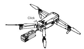
Removing the Intelligent Flight Battery
